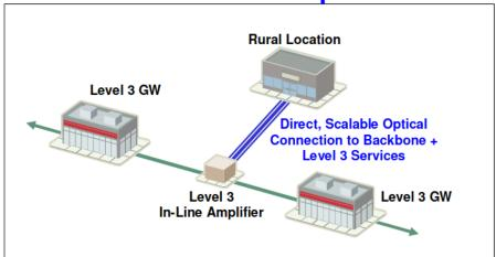
Level 3 proposes a solution to leverage its existing in-line amplifiers (ILA) to provide a lower cost, high bandwidth backhaul option for communities in underserved areas located near its ILA sites.
