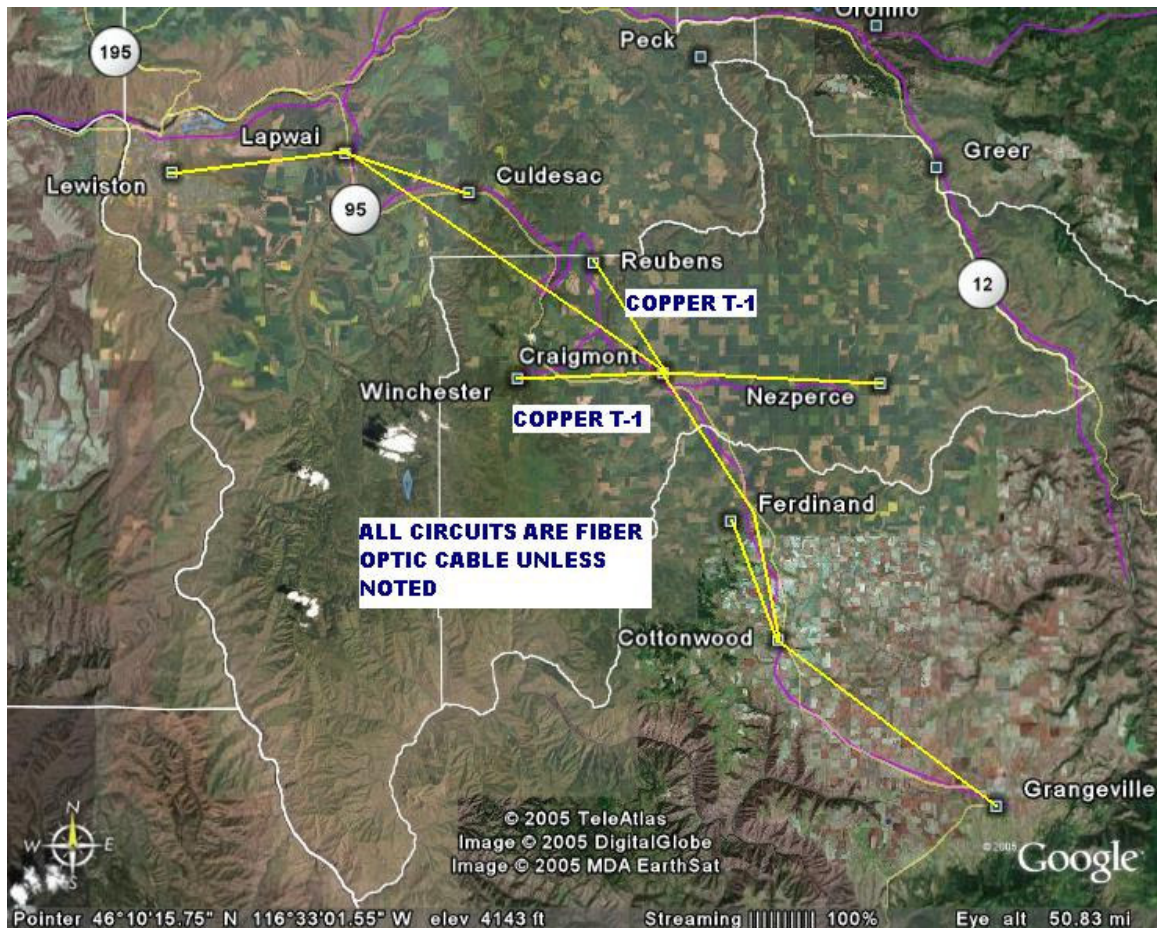
Figure 7. The Qwest network serves eight communities in the study and links most of the central offices with fiber optic cable.
