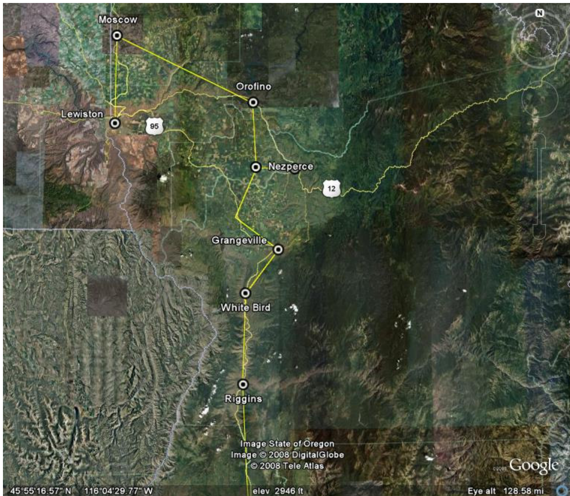
Figure 4. Final Phase One Schematic WAN Design (Yellow Lines). Note addition of Grangeville-White Bird-Riggins link to this phase.
