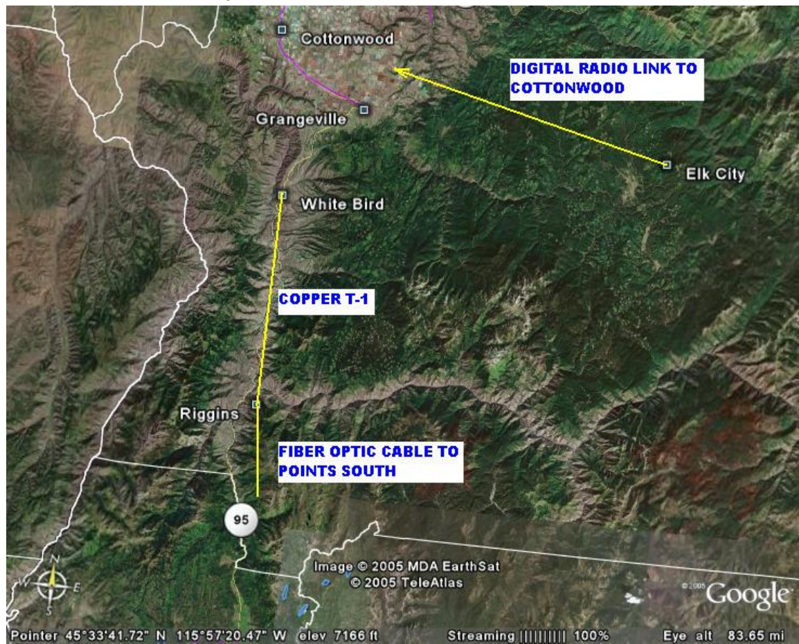
Figure 6. Frontier Communications serves three study communities with three different backhaul technologies.
