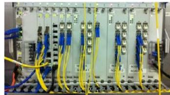
ICN uses the lab equipment above to test the configuration environment for the network prior to the deployment of equipment into the field.
