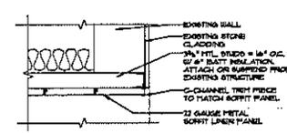
SOFFIT DETAIL SCALE: 1" = 1'-0"
