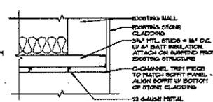
SOFFIT DETAIL SCALE: 1" = 1'-0"
